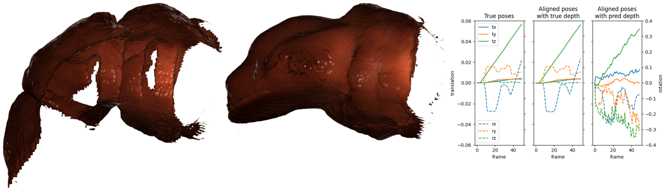
FIGURE 6 3D shape reconstruction results. The reconstructed shape from 50 frames of the true depth map (Left) and the predicted depth map (Middle), and the true poses and the estimated poses are compared (Right). The rotation parameters are in the axis-angle representation. Back faces are culled off for visualizing meshes.
