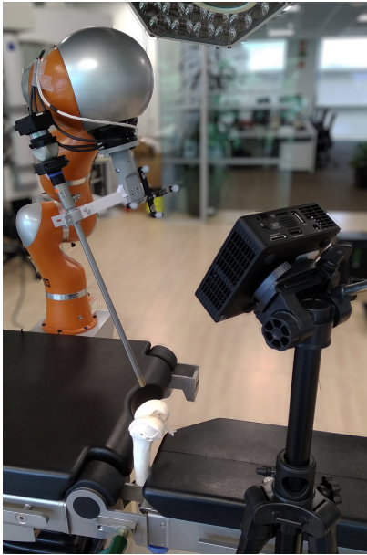
FIGURE 1 Left: Photograph of the proposed setup, including the robot-mounted endoscope, phantom and miniature projector. Right: schematic of the photogrammetric pipeline.
